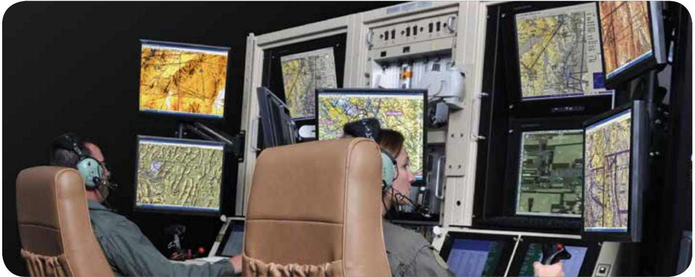
L3 Link Training & Simulation's Predator Mission Aircrew Training System (PMATS) is ushering in a new, advanced level of simulation to train pilots and sensor operators. PMATS consists of a form, fit and function interface for the pilot and sensor operator stations that uses ground control station hardware from General Atomics Aeronautical Systems, Inc., builder of the Predator and Reaper aircraft.
