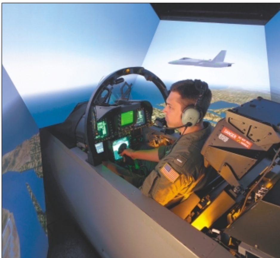
As part of the U.S. Navy's F/A-18 Super Hornet low-rate initial production program, L-3 Link Simulation and Training developed a new tactical flight trainer, using advanced visual technologies. (Boeing Company photo)
